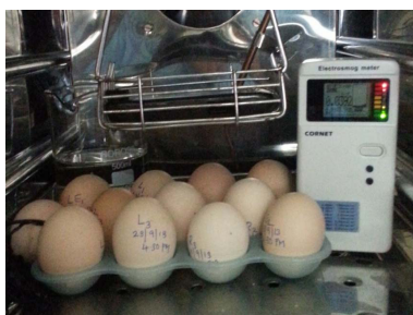
[Table/Fig-1]: A photograph showing the experimental set up. The Mobile phone (red arrow) is hung with a distance of 5 cm separating it from the fertilized chicken eggs. A RF meter is kept inside the incubator to check the intensity of radiation (yellow arrow).
